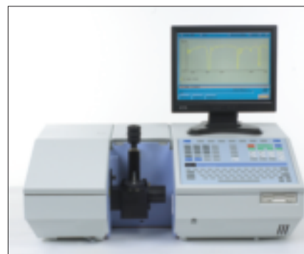
Figure 1. Spectrum RX I with single reflectance ATR.
